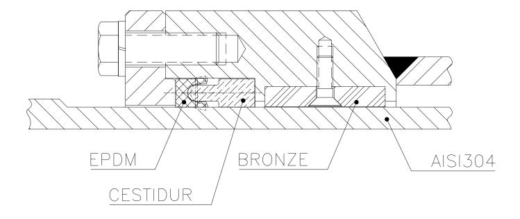
After changing the sealing replace the steel holding flange to its original position and tight all the holding bolts. It is recommended to tight the holding bolts in a "diametrical" way. Do not use sharpened tools during this process.
