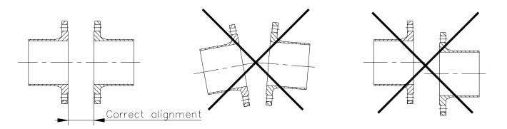
It is very important to ensure plainness and parallelism of the mating flange to avoid a leakage to the outside and avoid deformations of the valve.
